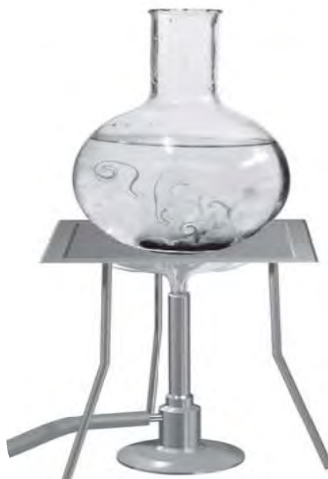
Fig.4.9: Convection of heat in water
