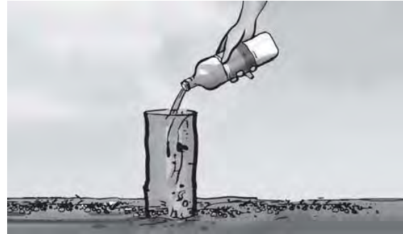
Fig.9.5 : Measuring rate of percolation
