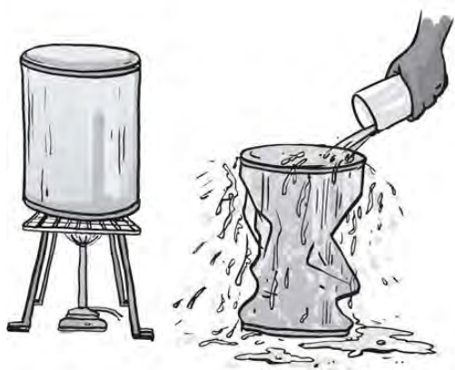
Fig. 8.2 : Can with hot water being cooled
