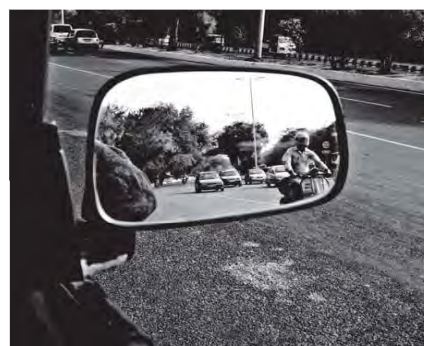
Fig.15.20: Convex mirror as side view mirror
