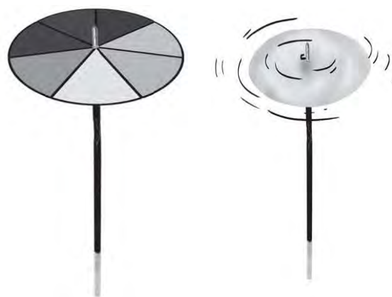
Fig.15.31: (a) A disc with seven colours (b) it appears white on rotating
