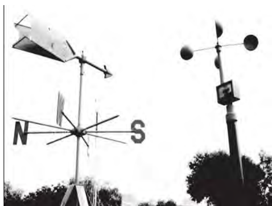
Fig. 8.17 : An anemometer for measuring the speed of wind Courtesy : India Meteorological Department, New Delhi
