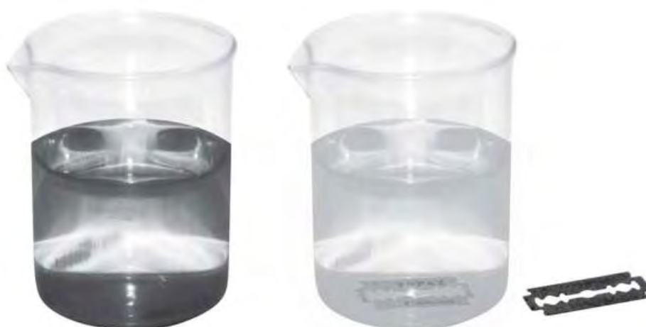
Fig.6.4: Change in colour of the copper sulphate solution due to reaction with iron
