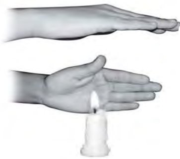
Fig.4.10: Transfer of heat by convection in air
